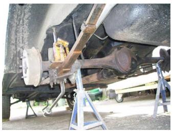
With that extra bit of clearance between the rear axle and the body, the new exhaust could easily be threaded over, taking care not to puncture the fuel tank, once in place it was just a case of hanging it on its supports and securing the manifold end with the clamp once a smear of exhaust sealer had been applied to the flange faces.
