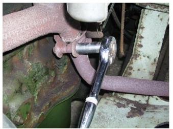
Removing the old one was easy once the manifold clamp was undone, it was that rotten that it could be snapped in three with almost no effort.
