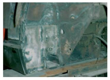
could be removed later) The off side was left in tact at this stage as it was the strongest side. The bottom edges of the A and B posts and bulkheads were all cleaned up, the new floor was tacked in place followed by the inner and outer sills, the remains of the rear suspension box was removed, the new rear spring mounting box was positioned on e the new floor and welded in place at the bottom, a repair section was made up and fitted into the
