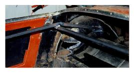
The bare shell was lifted up to a working height and supported on strong trestles that were set level, stiffening box sections were fitted between the bulkhead and upper rear body to keep things in line these were brazed in place, the doors were removed and more supports put in between the A and B posts. The car came with new outer sills, new
