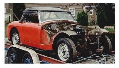
shell was complete with a free turning engine that looked correct, the doors opened and shut ok, the floor looked to consist of one patch on top of another, the boxes that hold the quarter elliptic rear springs were well rotted though still holding together, a bump in the area of the rear number plate had caused the rear boot section to bulge, the bonnet was solid but slightly miss shaped due to rot in the underside stiffening.
