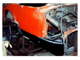
Small repair sections were made up and welded in where required, once all was fully welded top and bottom the stays
