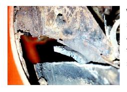
Work started on the near side, cutting out the sill and the floor, cutting away the bottom of the suspension box (the rest
