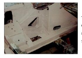
The inner wing sections had rotted in the triangle sections where road dirt had collected, rotten bits were cut out and replaced, the open area was also plated in to form a box section. The underside of the front cross member had been
